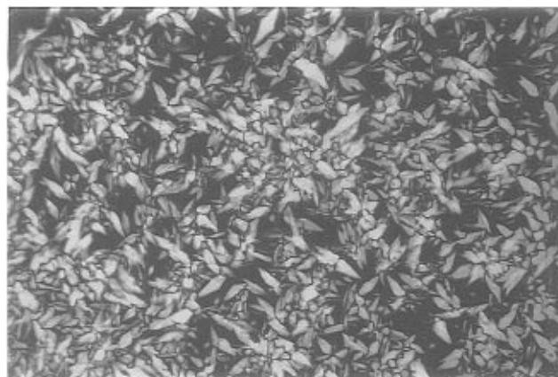
Figure 4. Texture of G1-(RF6) 12 at -17 °C observed between crossed polarizers.
